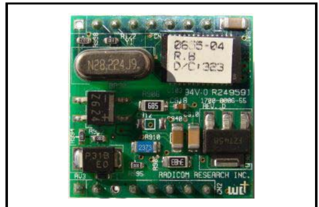
Figure 3-16 - Modem/Comm Card Mounting in E2
